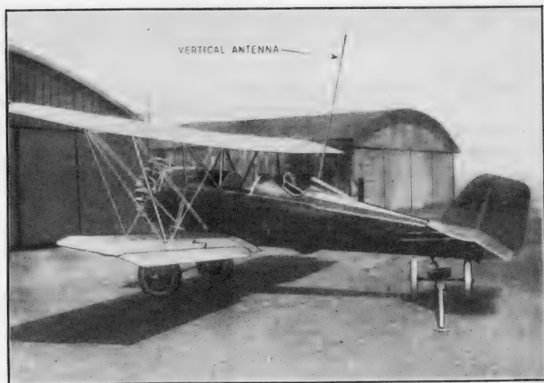
FIG. 447.—Showing how the vertical-pole type antenna may be installed on an airplane. This type antenna is usually employed for reception only.
