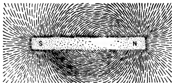
FIG. 1.—Lines of force and strain lines (magnetic spectrum) produced by a bar magnet as shown by the arrangement of iron filings.
