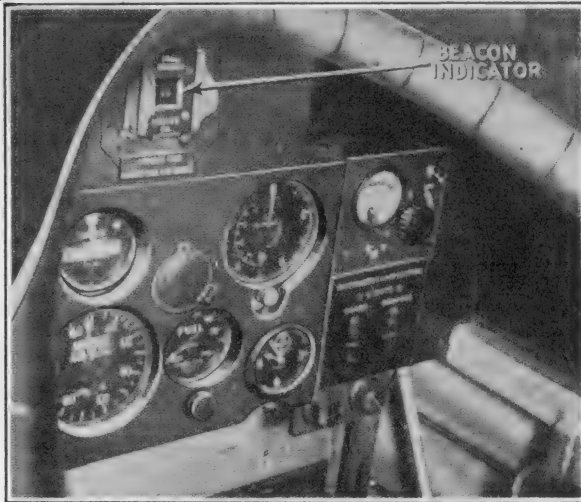
FIG. 431.—Showing a visual type radio beacon indicator mounted on the instrument board of an airplane, where it may be readily observed by the pilot.
