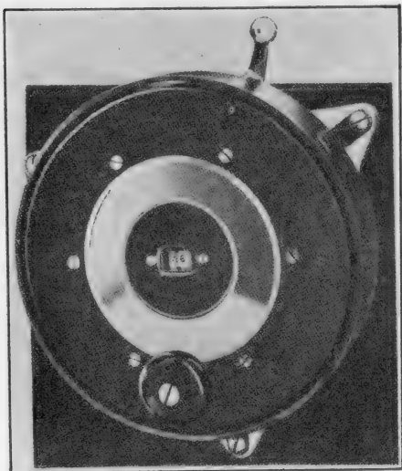
FIG. 450.—Insulated reel installed on aircraft for paying-out and drawing-in the trailing wire antenna—Western Electric type.
