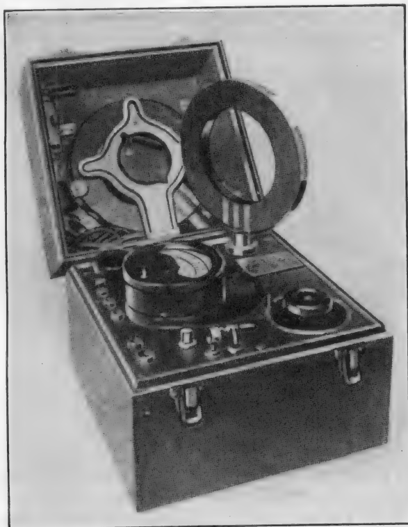
FIG. 304a.—The type D Kolster decremeter. One of the exploring coils is shown mounted in position.
