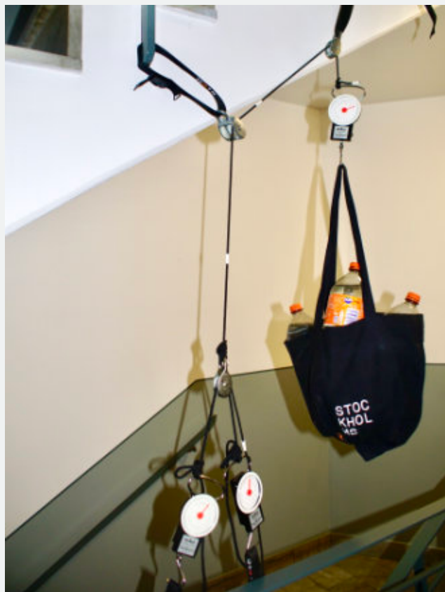
Exercise 2: Single block with pulling rope inserted in wall to gain power
