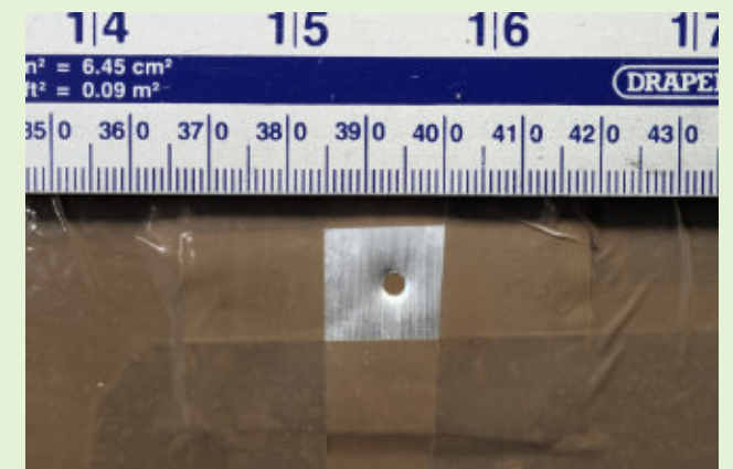
8. The pin-hole is about 3mm diameter
