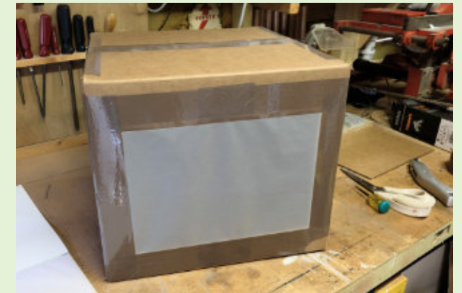
6. Tracing paper taped in place
