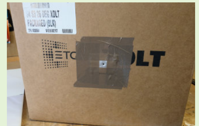
7. Pin-hole taped in place
