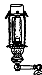
an incandescent mantle used with a gas burner (invented in Germany in 1890)
