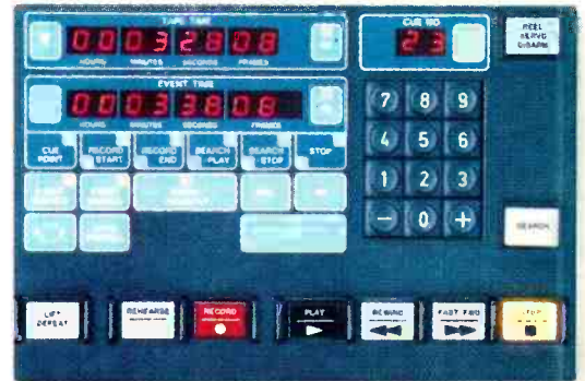
ATR-124's Multi-Point Search-To-Cue (MPSTC). Provides 100 cue locations.
