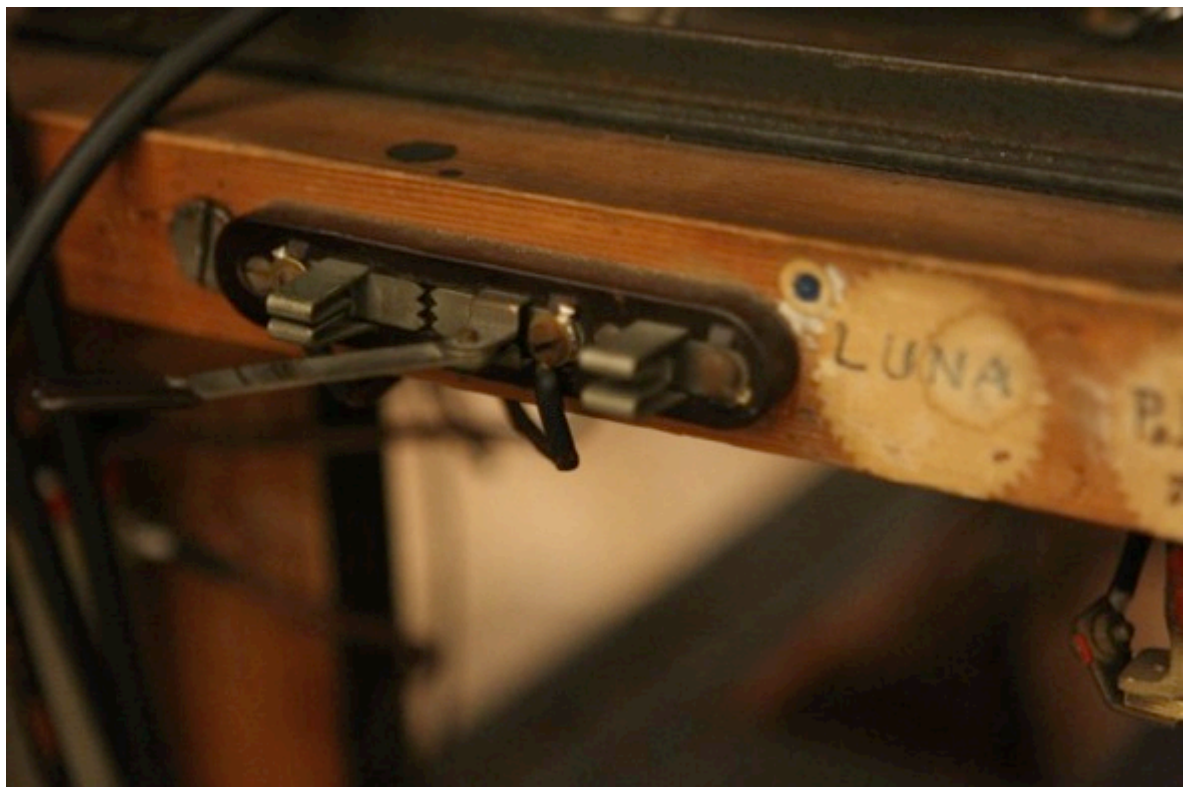
Fig. 86 Switch for the moon lamp on Fortuny's Bayreuth Theatre model. Photo Zeke Smith.
