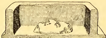
FIG. 5. MOULD FOR PLASTER OF PARIS CAST WITH FRONT WALL REMOVED
