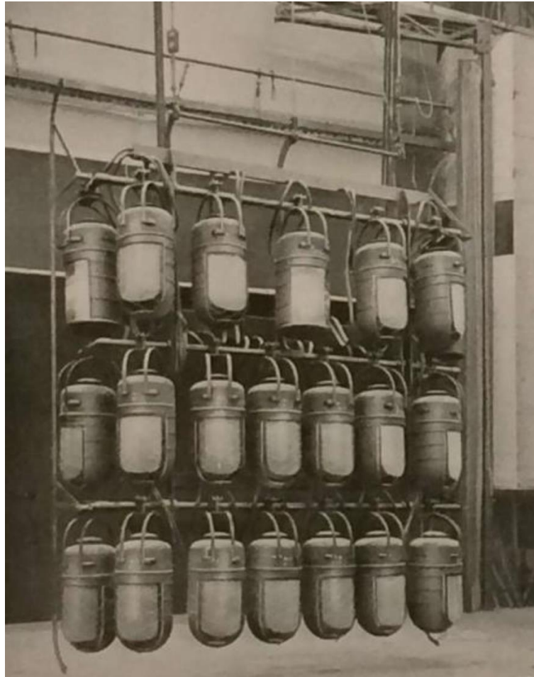
Figure 49. 20 cyclorama arc lights with rotating glass filters by Siemens, Künstler Theater, Berlin, 1913. (Johannsmeyer 1941)
