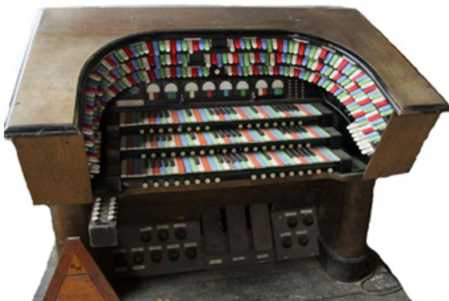
Strand Light Console with clutch-driven dimmers, Drury Lane, London c1950 Strand Light Console mit Kupplungsdimmern, Drury Lane, London um 1950
