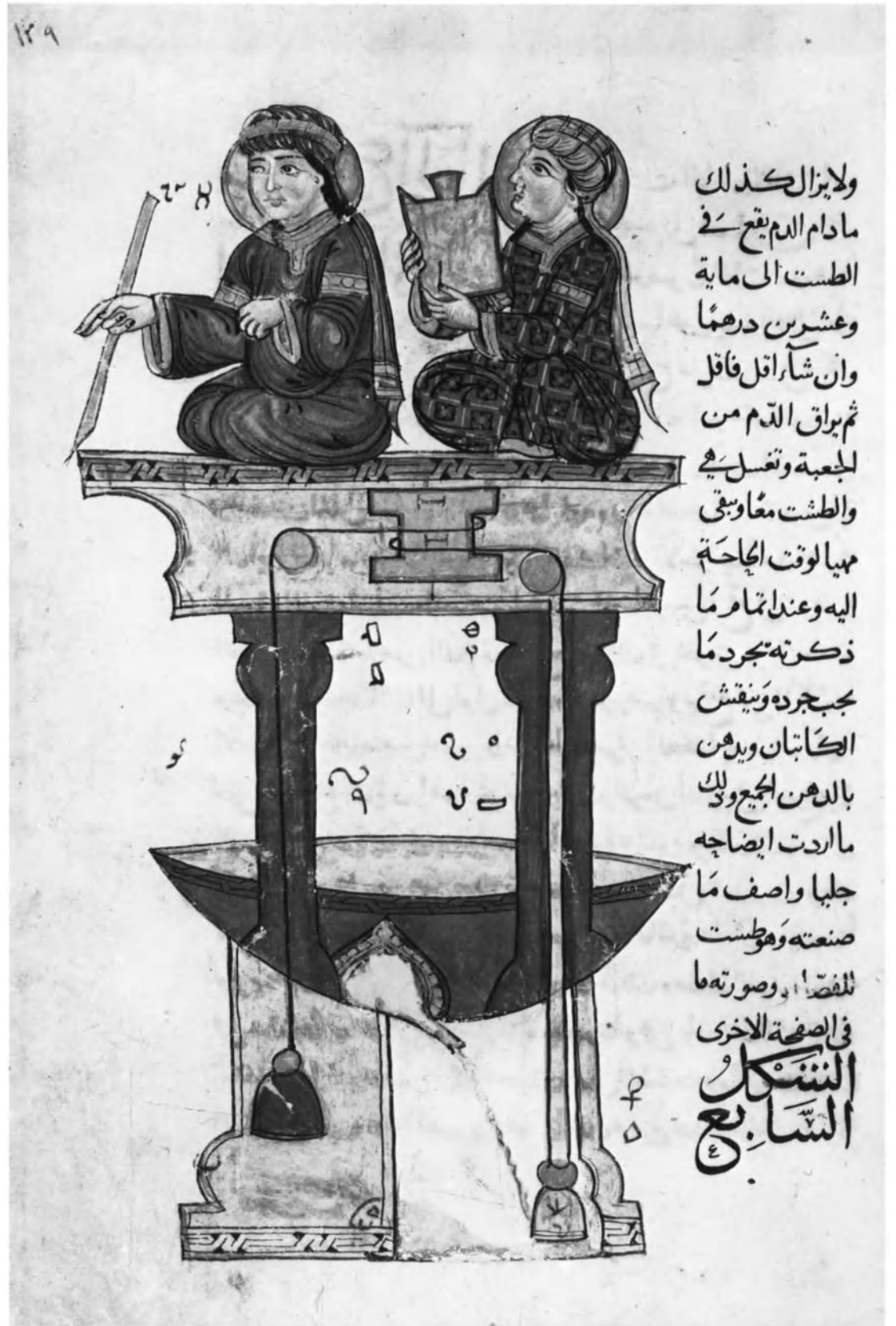
Plate XXII – 1315 MS. Main Illustration of Phlebotomy Measuring Device, Cat. III, Ch. 6. As Fig. 115. Courtesy of the Smithsonian Institution, Freer Gallery of Art, Washington D.C.
