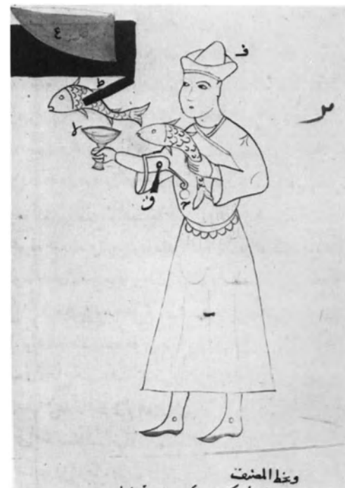
Fig. 98. Caption reads: And in the author's handwriting: 'I have drawn the bucket in its trough, and a pipe extends from it to the breast of the fish; on its end is a rod upon which it (i.e. the fish) moves and through which is the axle'.
