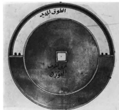
Fig. 20. Captions read: upper: 'the iron ring'; lower: 'the hole for the end of the axle'.
