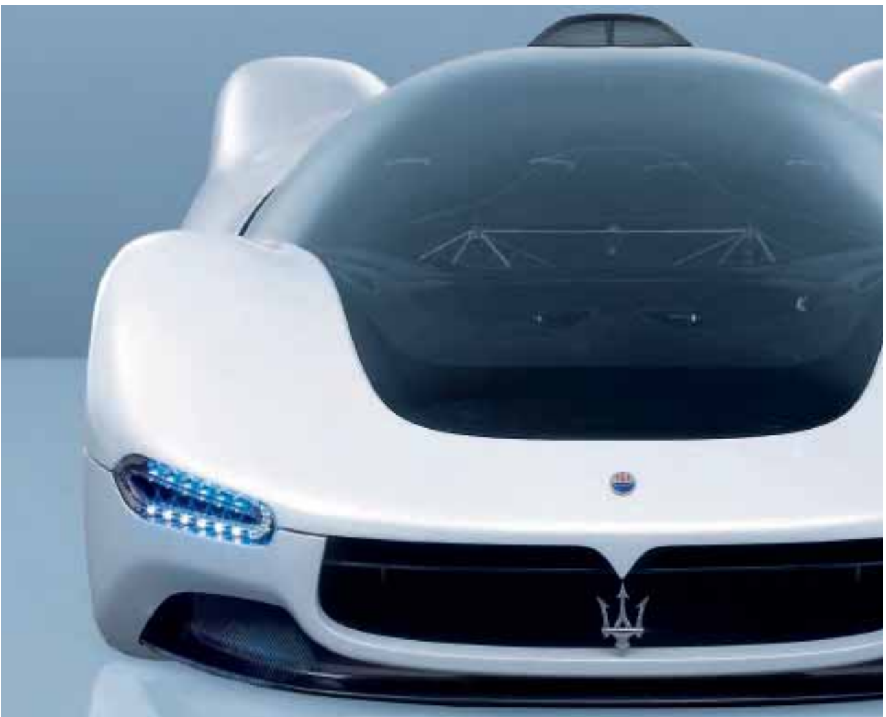
The automotive industry is using LED light as a major element in vehicle design. By 2010 the first approved models with LED headlights will be on the roads. There are already concept cars with these headlights, such as the Maserati Birdcage 75th which is equipped with OSRAM OSTAR® high-intensity LEDs.
