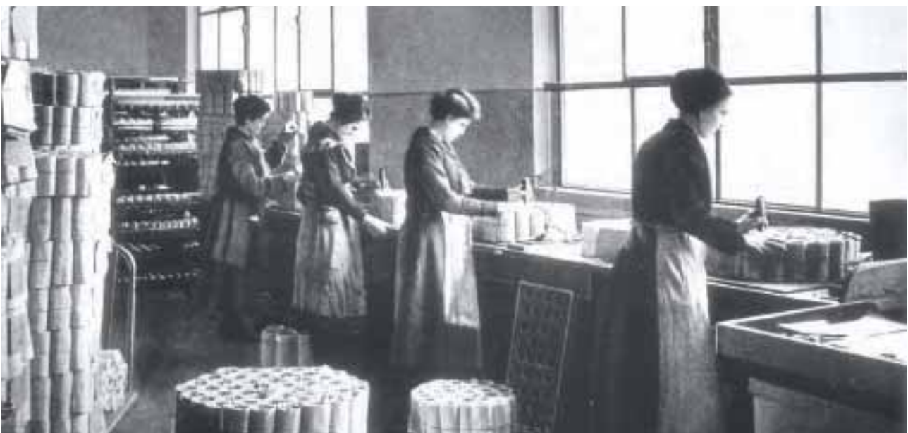
Testing the lamps before they are shipped from the factory has always been important. At the start of the 1920s this was an extremely time-consuming manual task.
