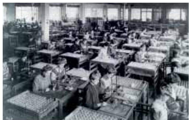
Base soldering was particularly labour-intensive.
