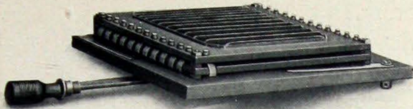
Figure 25—Early Ward Leonard Vitrohm Theatre Dimmer made up of two vitrohms rectangular plate units, connected together and mounted on a panel board which carried a dial switch with an extension lever to permit convenient adjustment. These dimmers were installed in Altmeyer's Theatre, McKeesport, Pa., in 1892.
