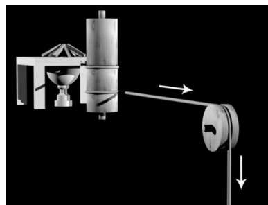
Figure 1.18 The mechanism for causing the fire representing Heron's torch to flare up. A cord attached to the counterweight, when pulled, causes, by means of a pulley, the vertical axle to revolve. This pulls a chain that removes a lid covering a small oil lamp, thereby allowing its flames to ignite wooden shavings that have been placed upon it. The fire is then viewed through an aperture cut into the architrave or pediment of the theatre box
