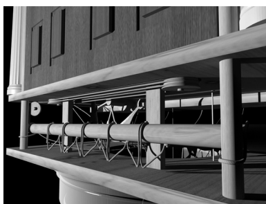
Figure 1.8 View under the stage showing the mechanism which controls the opening and closing of the stage doors. Above the horizontal rod operating this is the system of cords and pulleys which cause the figure of Athena to stand, move around the stage on a track, and then recline again
