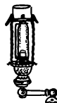
an incandescent mantle used with a gas burner (invented in Germany in 1890)
