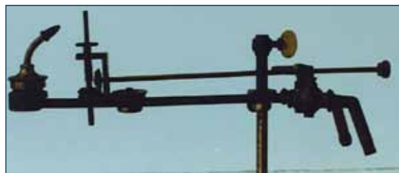
Fig. 3 Left: a Drummond lamp at the Collège Saint-Marc in Alexandria (Egypt), manufacturer unknown. Right: 'horizontal' Drummond lamps. Top: Queen's College, Belfast (N. Ireland), manufacturer: Yeates, note the platinum nozzle for use with hydrogen. Down: a beautiful model made by J. Salleron (Paris, 1869), Teylers Museum, Haarlem (The Netherlands).
