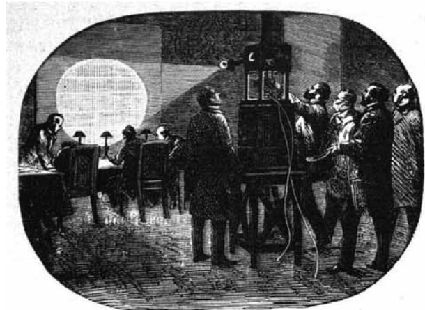
Fig. 6 But what are those people doing? The picture shows a projection of microscopic dispatches during Paris siege by the Prussian army, 1870-1871. The collodion microfilms were sent by pigeon post over the enemy's lines. The projection lamp was either a Drummond light (here, as revealed by the two feeder pipes) or a regulated electric arc (Duboscq 1885, p. 16).
