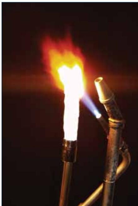
Fig. 1 The 'quicklime effect': an image today, of a Drummond light obtained by violently flaming a piece of quicklime with a modern blowtorch. Foreground: the concentric nozzle of an original lamp, of course not in service.
